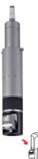
Precision at a 45-degree angle - this tool can cut it! Especially for mat-cutting applications, clean, precise 45-degree bevel cuts are essential. Relative cutting mode (to the surface of the material) guarantees a high degree of depth control. The maximum material thickness for this tool is 5mm (3/16").
