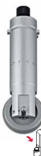
The crease tool type 1 is designed specifically for creasing multiple-wall corrugated cardboard and plastic materials up to thicknesses of 7mm/1/4". The large diameter of this type of crease wheel permits creasing of thicker materials cleanly and with considerable down pressure, without breaking or tearing the top sheet.
