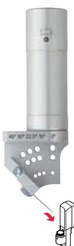
The seemingly impossible made nearly commonplace: 3D structural designs with the V-cut tool. This unique tool is ideal for cutting extremely rigid sandwich board materials. Five different angles (0°, 15°, 22.5°, 30°, 45°) are possible. Depending on material density, thicknesses of up to 16mm/5/8" can be processed.
