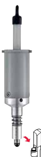
The raster method has emerged as the preferred method for producing tactile Braille signage for the blind and visually impaired. The Braille tool is fully compatible with both the G3 Universal Module and the PN-series TZ-modules. The process is quite simple: a router module routes the holes, and the Braille tool inserts balls to create raised dots.
